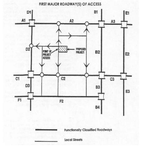
Roadways A, B, C, D, E, and F are all shown on the Functional Classification Map. Subscripts indicate segments, or links, comprising parts of each functionally-classified roadway. Extent of each link (e.g., B2) is determined by defining points of intersection of two or more functionally-classified roadways indicated by a square ( $\Box$ ).
